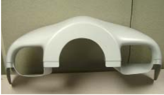
Figure 3. Carbon fiber upper nose bowl. (Courtesy of Atlantic Aero.)
