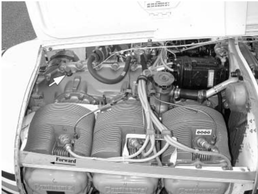
Figure 1. Teledyne Continental IO-520BB engine installed in the test aircraft.
