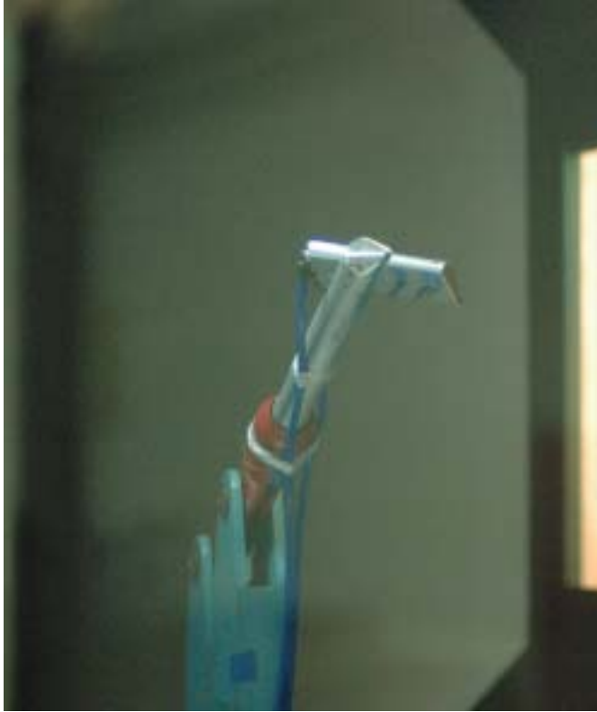
Figure 13. Angle of attack probe pitched 25^\circ , yawed 10^\circ and rolled 45^\circ . The viewpoint is directly into the image.
