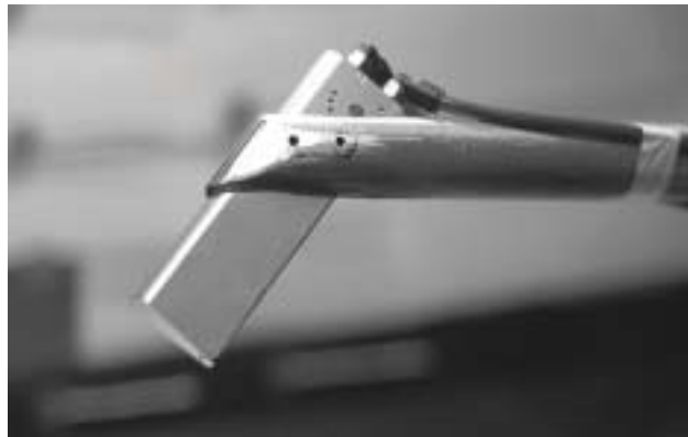
Figure 3. Angle of attack probe mounted in the wind tunnel.
