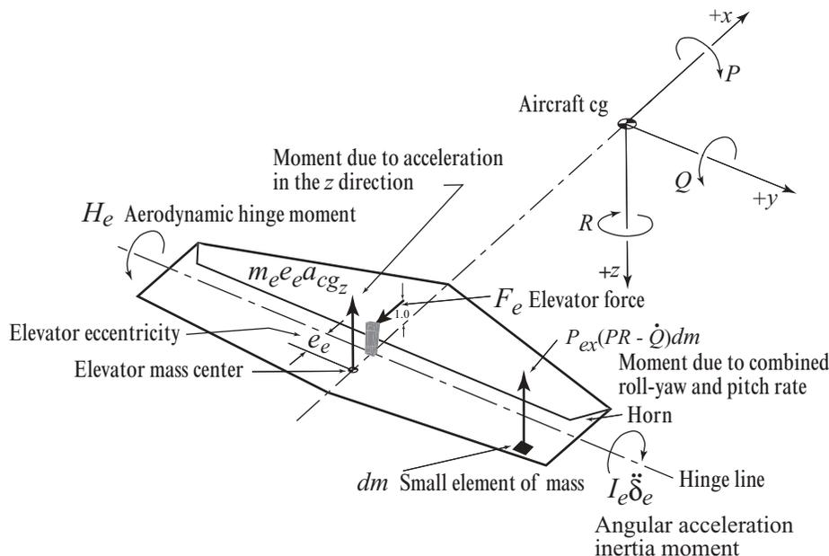
Figure 1. Elevator schematic
