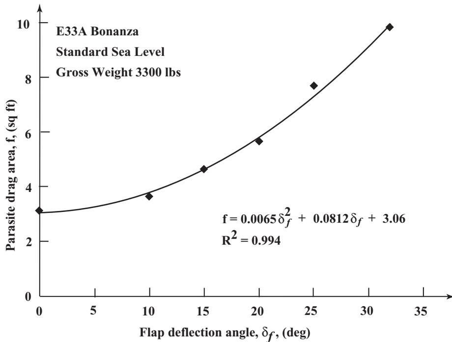
Figure 3. Equivalent parasite drag area as a function of flap deflection angle,  $\delta_f$ .
