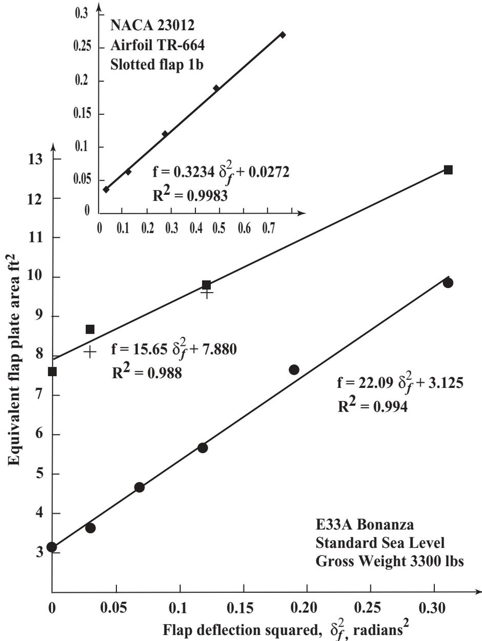
Figure 4. Equivalent parasite drag area as a function of the square of the flap deflection angle,  $\delta_f^2$ .
