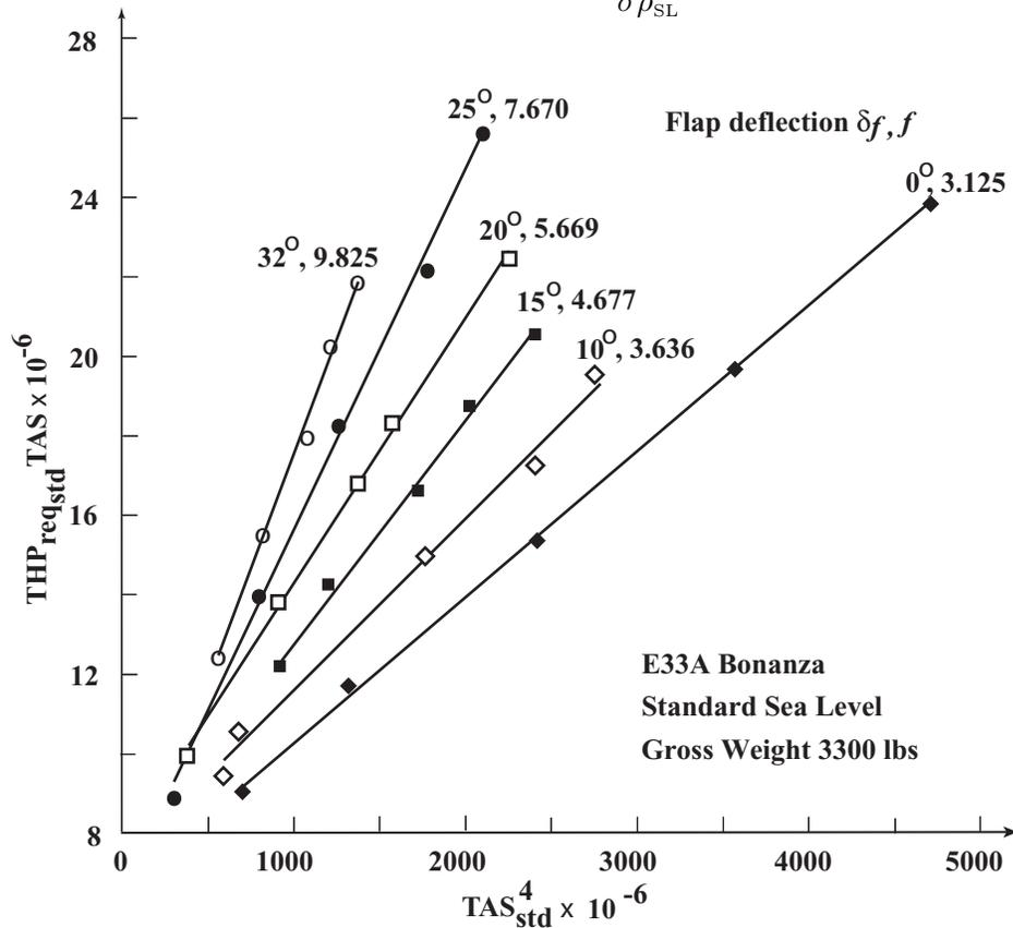
Figure 2. Equivalent parasite drag area for various flap deflections.
