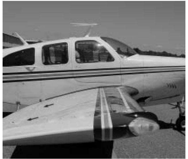
Figure 4. Vortex generators installed on wing.
