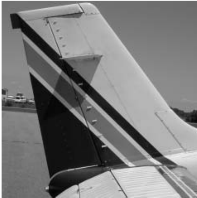
Figure 3. Vortex generators installed on vertical tail.
