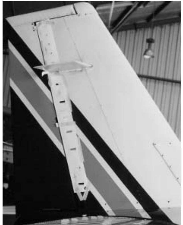
Figure 2. Vertical tail installation templates. VGs layed out on the horizontal tail for installation on the vertical tail.
