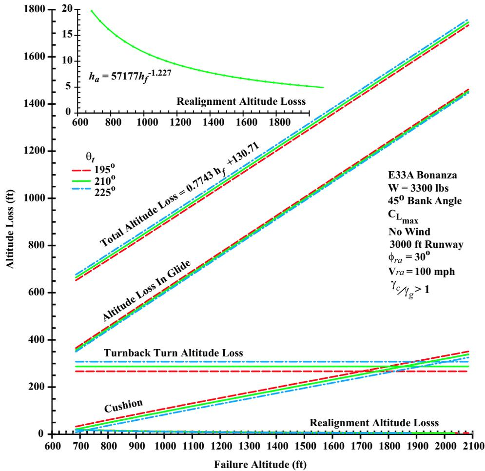
Figure 11. Altitude loss for an E33A Bonanza for various turnback turn angles for a 3000 ft runway.
