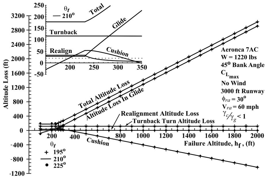
Figure 15. Altitude loss for an Aeronca 7AC for various turnback angles for a 3000 ft runway.
