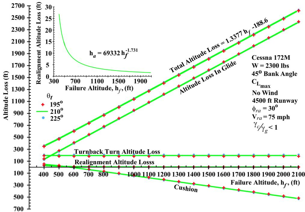
Figure 13. Altitude loss for a Cessna 172M for various turnback angles for a 4500 ft runway.
