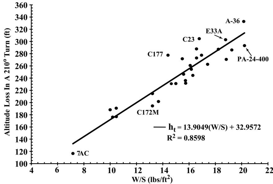
Figure 19. Altitude Loss,  $h_t$ , in a 210° turnback turn at  $C_D/C_L^2$  vs wing loading  $W/S$
