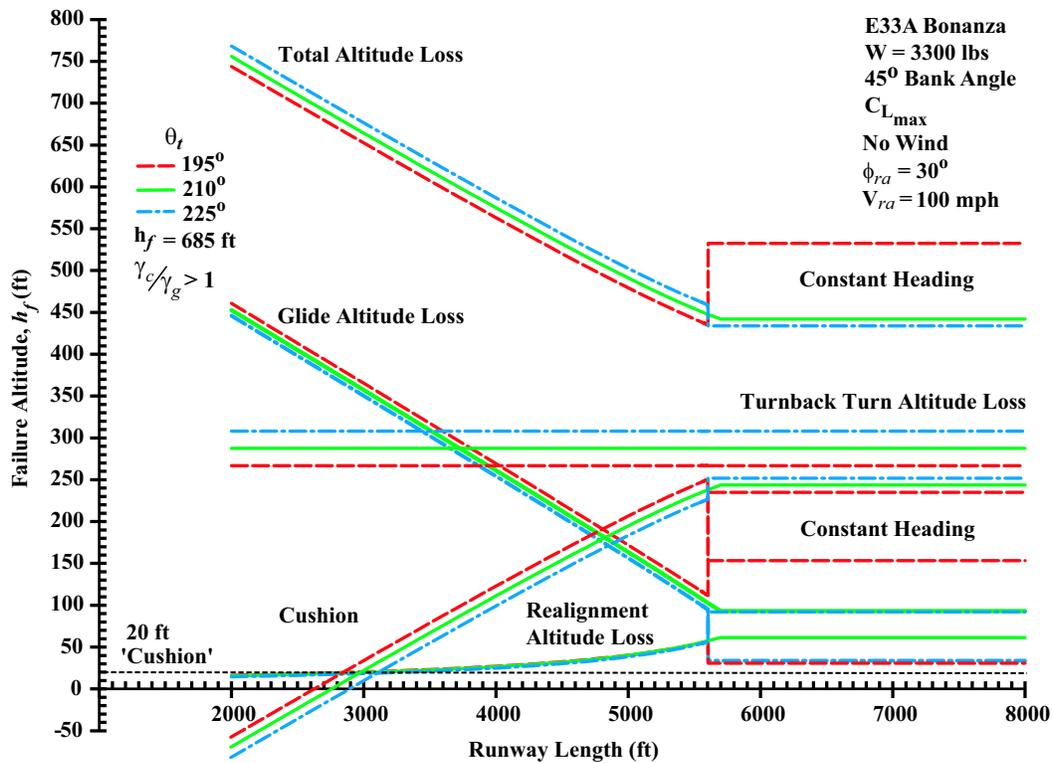
**Figure 12.** Altitude loss for an E33A Bonanza for various turnback turn angles and runway lengths for a 685 ft failure altitude.
