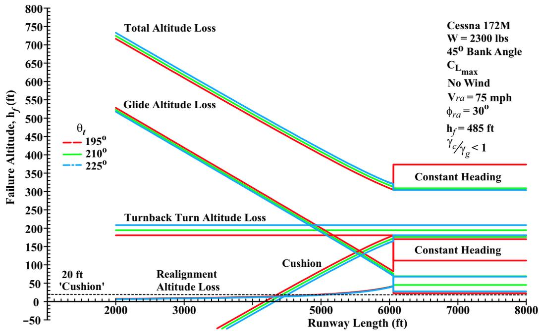
Figure 14. Altitude loss for a Cessna 172M for various turnback turn angles and runway lengths for a failure altitude of 485 ft.
