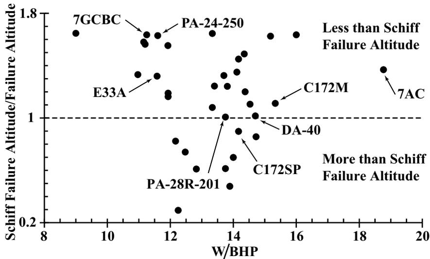
Figure 23. Schiff  $1\frac{1}{2} \times 360^\circ$  turn failure altitude ‘rule of thumb’ compared to the estimated failure altitude,  $h_f$ .
