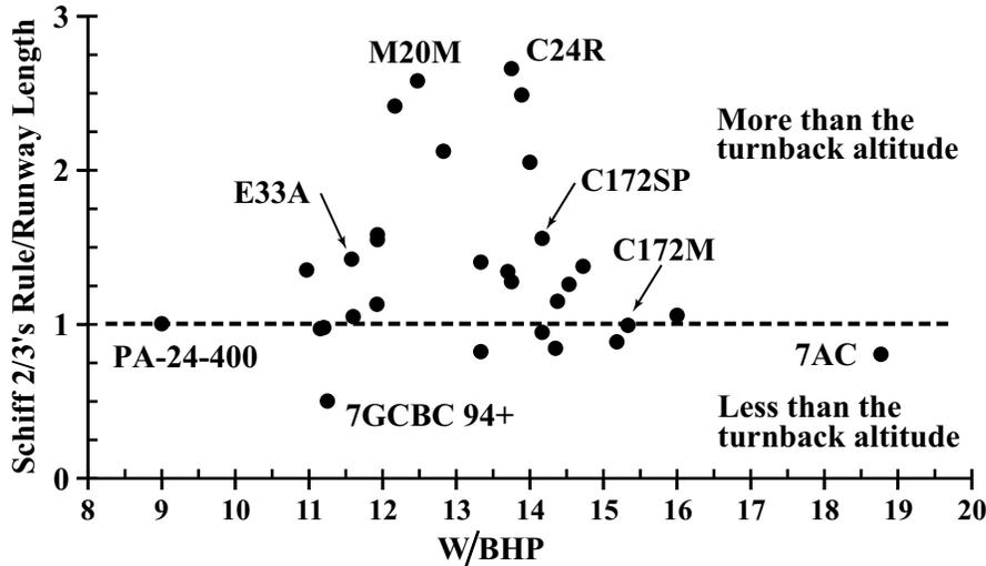
Figure 24. Schiff two thirds ‘rule of thumb’ compared to the estimated runway length.
