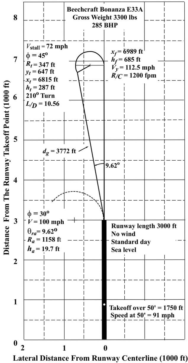
Figure 4. Scaled turnback diagram for an E33A Bonanza.
