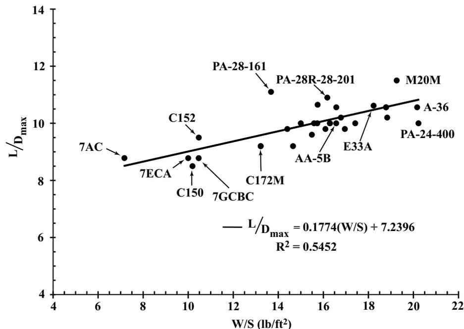
**Figure 22.** The effect of wing loading  $W/S$  on  $L/D_{\max}$ .
