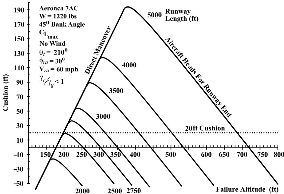
Figure 16. Cushion versus failure altitude for an Aeronca 7AC for various runway lengths.
