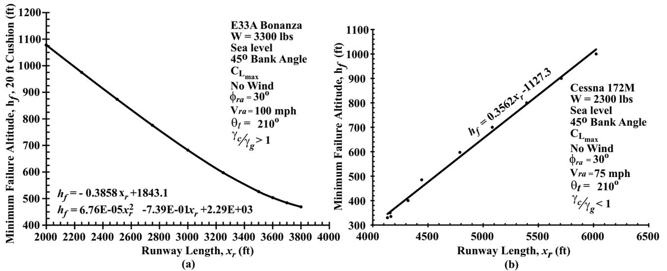
**Figure 7.** Comparison of the minimum failure altitude for an E33A and a C172M when the aircraft heads for the runway end.
