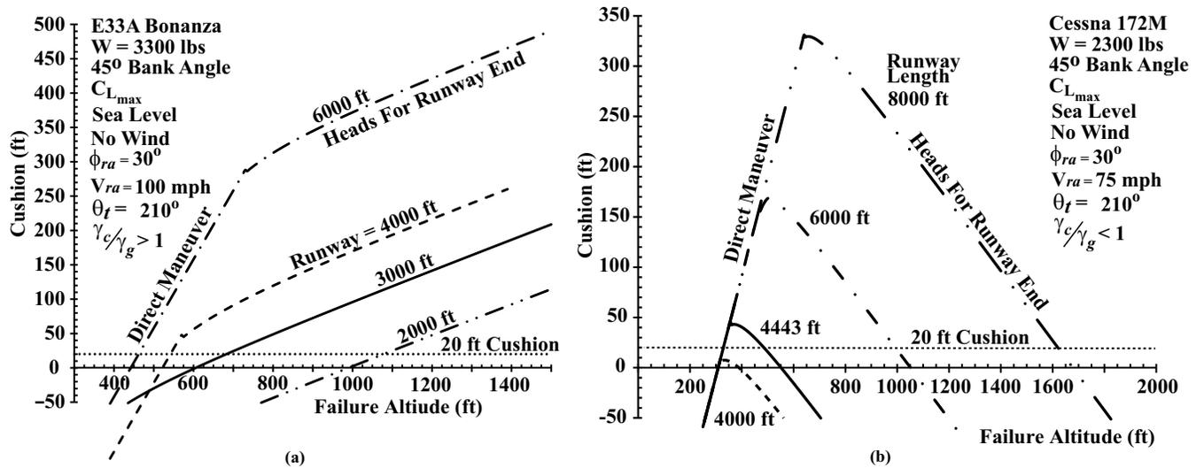
**Figure 8.** Comparison using 20 ft cushions for an E33A and a Cessna 172M for various runway lengths.
