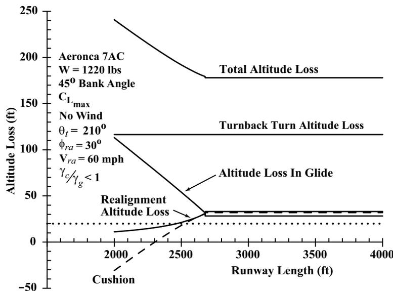
Figure 17. Altitude loss for an Aeronca 7AC for  $h_f = 210$  ft and a turnback angle of 210°.
