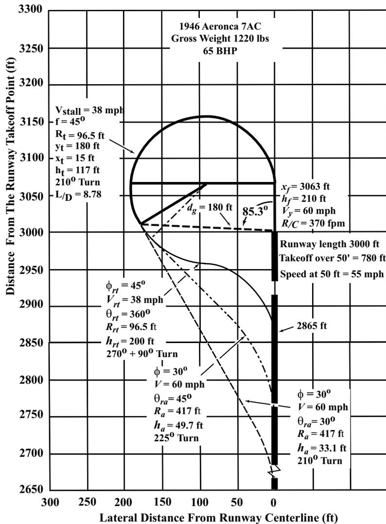
Figure 10. Scaled turnback diagram for an Aeronca 7AC: failure altitude 210 ft, runway length 3000 ft, 270° turn at  $C_{L_{max}}$ , bank angle 45° followed by a reverse 90° turn also at  $C_{L_{max}}$  and a bank angle of 45°.
