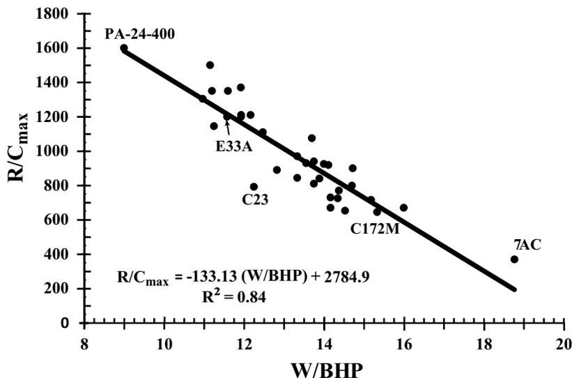
Figure 18. Maximum rate of climb,  $R/C_{max}$  vs power loading  $W/BHP$ .
