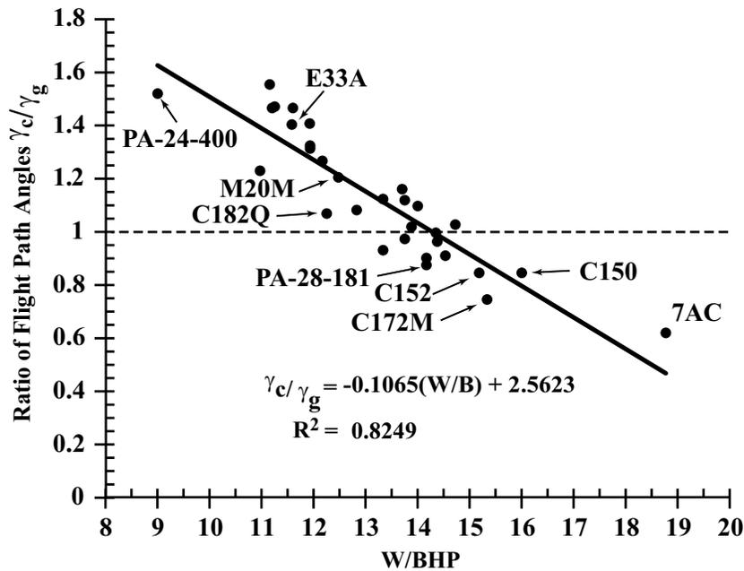
Figure 21. The effect of power loading  $W/BHP$  on  $\gamma_c/\gamma_g$ .
