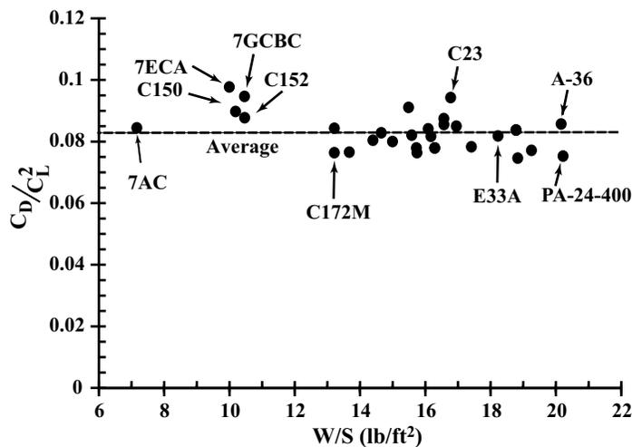
Figure 20.  $C_D/C_L^2$  in a 210° turnback turn vs wing loading  $W/S$ .
