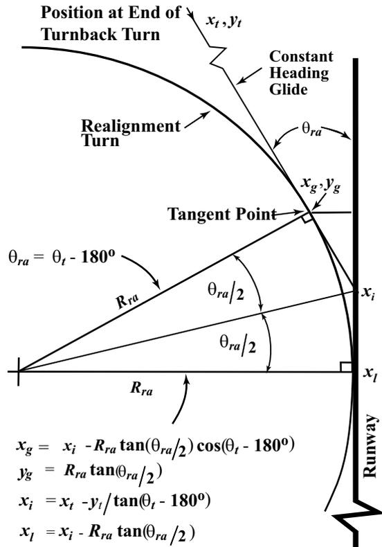
Figure 2. Direct heading geometry.
