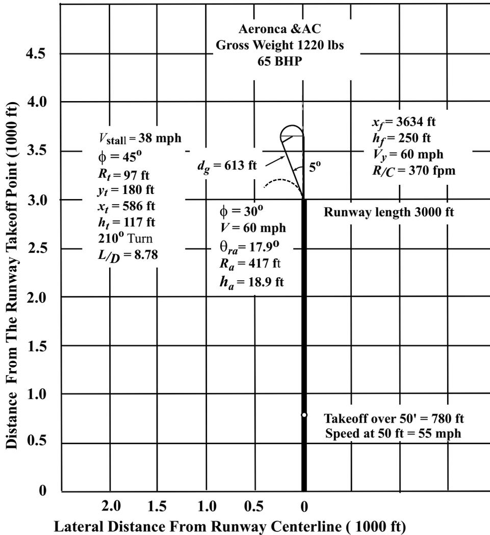
Figure 9. Scaled turnback diagram for an Aeronca 7AC: failure altitude 250 ft runway length 3000 ft.
